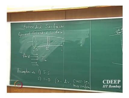
When a general arbitrary shape, let us assume that this is the varying cross sectional system and we are going to take specific examples and specific cases of this generalized a generalized pin to extended surface. So, if we want to quantify heat transport process in such a generalized system we need to write a we need to find the temperature distribution and in order to find the temperature distribution we need to write the energy balance that is what we have been doing.
