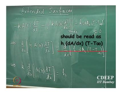
So, far now, I could rewrite this as d by dx k A of x dT by dx equal to d by dx h s into T minus T infinity. So, if I assume that the thermal conductivity and the heat transport coefficient are not function of position then one could pull it out and say k d by dx A of x equal to h is T minus T infinity a function of position in this term here yes or no.
