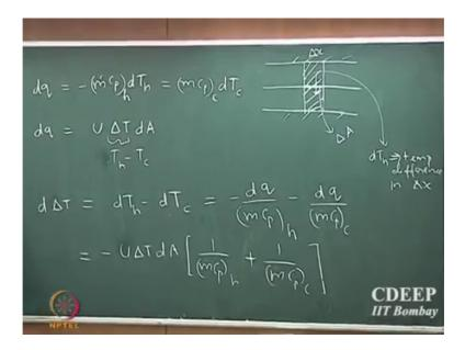
So, we are going to write a simple energy balance. So, here is the parallel flow, I take a small element. So, supposing if it is delta x some whatever small element and let us assume that the area of heat transport in that element ok. So, this area is delta A so, that is the area of heat transport which is available for taking heat from the hot fluid to the cold fluid.
