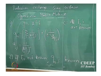
So, the total emission from all the surfaces was just the solution of this matrix problem right. So, J will be A inverse times b ok. So, where if I open up the A matrix a 1 1 the first element in the matrix will be sum over all j 1 by A 1 F 1 j inverse plus 1 by 1 minus epsilon 1 divided by A 1 epsilon 1 so that will be the first term.
