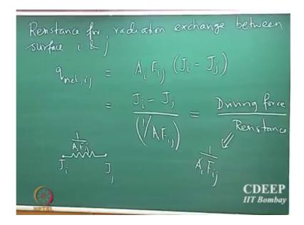
So, radiation exchange between surface i and surface j is given by is Ai Fi j into j i minus j ok. So, now we can rewrite this as Ji divided by 1 by Ai F ij. So, if the driving force for radiation exchange is the difference between the corresponding total emission from each of these surfaces so that is the driving force, driving force divided by the resistance ok.
