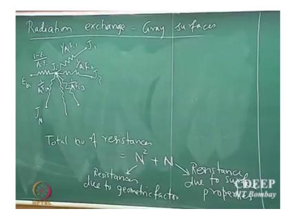
So, supposing E bi is the blackbody radiation for surface i and J i is the corresponding total emission from that surface then the resistance offered is 1 minus epsilon i by Ai epsilon ok. Now this is exchanging radiation with all other surfaces therefore, you have resistance for which are occurring in parallel, because it is simultaneously exchanging radiation with all other surfaces.
