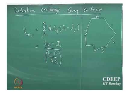
We looked at the energy balance or radiation exchange in gray surfaces. So, we said that the net radiation exchange, if we have an enclosure with N objects with N surfaces and each of them are exchanging radiation with each other. Then we said that the net radiation exchange is given by sum over all Ai F ij, j going from 1 to N and that is also equal to E b i minus J i by 1 minus epsilon i by Ai epsilon ok.
