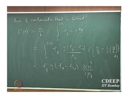
How do we relate the amount of condensate to latent heat? The amount of heat; so, we are going to write a simple heat balance. So, this is my wall (Refer Time: 00:26) film.
