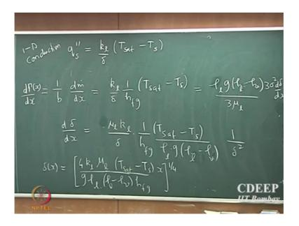
So, remember that now, it is a 1 D conduction problem ok. So, it is a fixed temperature the temperature of one end of the 1 D problem is T s and other end is T sat ok; q s is simply given by k liquid that is the conductivity of the liquid divided by delta; divided by the thickness of the 1 D slab right multiplied by T sat minus T s that is the flux of heat transport ok.
