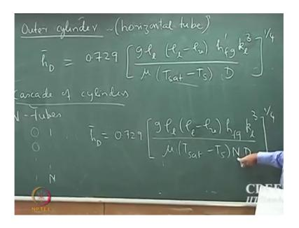
So, that is a place where the condensation crosses at the exterior of the cylinder or the curved surface of the cylinder plays and important role. So, these kind of correlation are actually very commonly used in the heat exchanges at the; so, the correlation. So, that is outer cylinder and it is a horizontal tube.
