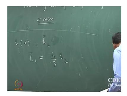
So, now, he said there are two objects one is the local heat transport coefficient and second one is the average heat transport coefficient ok. So, suppose is the length of the plate is L.
