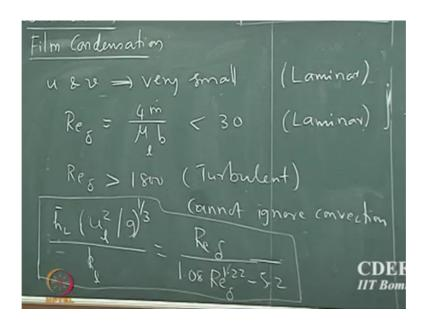
So, when we started this discussion we said that u and v are very small right. So, what will be the nature of the flow if u and v are very small? Small velocity? Come on velocity is small what is the nature of the flow? Is laminar right so what we looked at is laminar condition. So, one could also have turbulent condition for the same problem and so, the Reynolds number.
