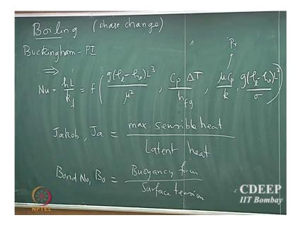
So, that will be Nusselt number equals to hL by kf and there will be a function of g rho l rho v, L cube by mu square comma C p delta T by and mu C p by k which is Prandtl number l square by sigma what is C p delta d by hfg? Hfg is the latent heat. So, that tells you.
