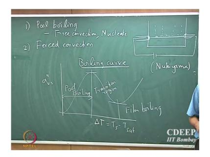
So, that two classes of boiling, one is called the pool boiling and the other one is called the forced convection boiling. So, it might be a bit surprising to see forced convection here. So, we will see that although the fluid is not being pumped or it is not being forcefully made to flow towards something, that you will see that there is a certain type of forced convection which is involved and we are actually discussed very deeply when we go to that topic ok.
