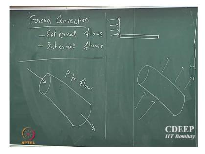
And that could be different geometric, it could be a flat plate it could be a cylinder. It could be inside the cylinder etcetera. And the other one parallel is the natural convection, which we will see after completing the forced convection topic. So, here you can have 2 types. One is the external flows, and internal flows. You have 2 types. So, external flow very simple example of that is you have a flat plate, in you have fluid which is flowing faster this flat plate, that is an external flow.
