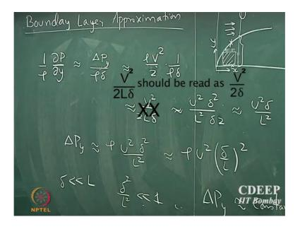
So, d P by d y. So, suppose, the suppose if delta P is the pressure gradient in the y direction. So, delta P y, this will scale as RHO into delta. So, y direction scales as the boundary layer thickness now delta P y. So, that is the. So, delta P y is given by the inertial. What are the pressure terms in terms of velocity? How do we write pressure delta P in terms of velocity?
