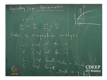
So, we stopped in the last lecture by looking at the gradients in the boundary layer. So, we introduce the boundary layer approximation, where we said that x component velocity is much larger than the y component velocity and we said that d u by d y is actually larger than d u by d x and d v by d y is larger than d v by d x. Note that I made a typo this should be x and not this should be y and not x.
