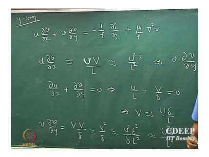
If you look at the y component momentum balance, you will have u d v by d x plus v d v by d y that should be equal to minus 1 by rho d P by d y plus mu by rho into del square v. So, that is the y component momentum balance. Now, the order of magnitude of u is the free stream reference velocity. So, u d v by d x would actually scale as u that is the order of magnitude for the x component velocity multiplied by v, which is the order of magnitude for the y component velocity divided by l.
