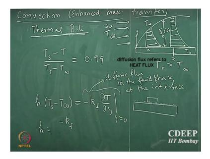
So, therefore, the there has to be something called thermal boundary layer, very close to the interface there will be a thermal boundary layer. So, supposing if the temperature of the flat plate is let us say T s and the temperature of the free stream fluid is T infinity, now there is going to be a boundary layer. So, that is the thermal boundary layer. If I assume that T s is greater than T infinity what will be the temperature profile.
