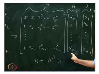
This can be simply transformed into 1 z1, z1 square z1 raise to n 1 z2 z2 square z 2 raise to n. So this is simply solving Ax=b. Well unfortunately life is so simple because it turns out that if you want to develop a higher order interpolation polynomial nth order interpolation polynomial in general about 3 or 4 this matrix here it looks very simple right Ax=b. This is known to you these values are known to you function values are known to you right now.
