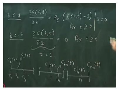
Sorry this is not 1 this is t. So this boundary condition is at z=1, this boundary condition is at z=0, so the solution now, solution now is actually function of 2 independent variables, one is time one is space and other is time. At z=0 for all time this boundary condition will hold at z=1 at z=1 at all time this boundary holds, okay. I want to know discretize this particular problem using finite differential method. Okay. Using finite difference method.
