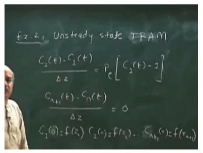
So what will be here. C2 t-C1 t/delta z. I am taking forward difference approximation here. And =peculate number into C1 t -1, so this is one algebraic equation. Okay. What is the second algebraic equation? So what I get here is the differential algebraic system. Okay. I got differential equations in time and I got 2 algebraic equations. Actually this is a simple problem in this particular problem I can eliminate 2 variables.
