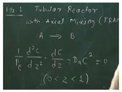
So my first example is going to be a Tubular Reactor example. So my first example is TRAM or Tubular Reactor with Actual Mixture. I am going to just take the equations and then we will see how to discretize, that is the key thing here. So this is the simple reaction where A goes to B, okay. A very, very simple reaction where A goes to B. And the ODE BVP that is given to you is 1/Peclet number \* d2c/dc square/dc/dz – this is Damkohler number \* c square = 0.
