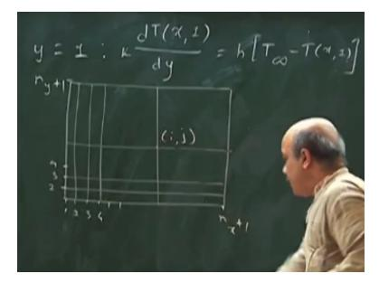
So I have convectively transferred at the 4th boundary at y=1 I have k. Okay. So I have 4 boundary conditions here. I have 4 boundary conditions here. Okay. Now how may I be going to discretize this? I am going to use Taylor series approximation in one dimension at a time. So I am going to I am going to discretize this domain okay by constructing grid points, now my domain is something like this.
