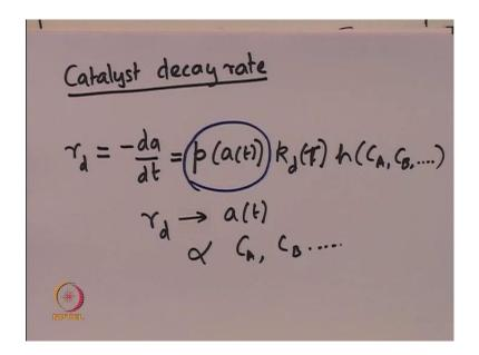
So, the decay rate typically takes the same form as that of the rate law. So, therefore, the decay rate r d is given by is minus da by dt that reflects the rate of change of activity, which respect to time. This should be equal to some function p, which depends on the activity itself multiplied by the corresponding specific decay constant, which depends which is a function of temperature multiplied by some function of concentration of all the species.
