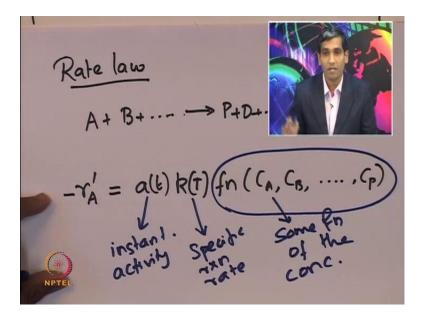
So, suppose if the catalytic reaction is A plus B plus gives P plus D plus. So, now, we can write the rate of consumption of species A because of catalytic reaction as the product of activity of the catalyst multiplied by the corresponding specific reaction rate,
