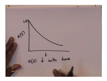
The typical profile, it starts with one because it is a fraction and it is a fraction of catalyst that activity which is left and so it goes from it exponentially decreases with time. So, clearly a of t decreases with time; so suppose if there is a reaction, how do we write the reaction rate law when there is catalytic deactivation process occurring simultaneously.
