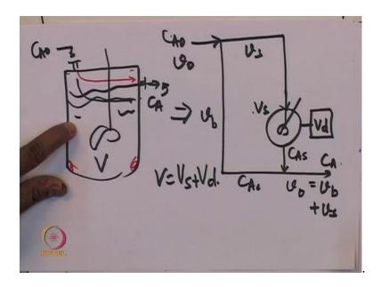
So, I made tree this particular reactor this is my real reactor equivalent to something like this see bypass means, it is not spending time in the reactor at all they would just it is going out. So, bypass is directly going out that means, not spending time in the reactor; whereas, some part is remaining here dead zones which is not seeing turbulence at all. So, I can look at this particular reactor as a set or network like this.
