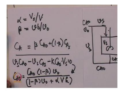
So, same figure now that balance this 1 CA I will right expression for this now before, so let me as let me say that alpha is equal to Vs by V0 what is Vs? Vs is the volume of this reactor and what is V is the total volume that is the alpha is a fraction of volume which is
