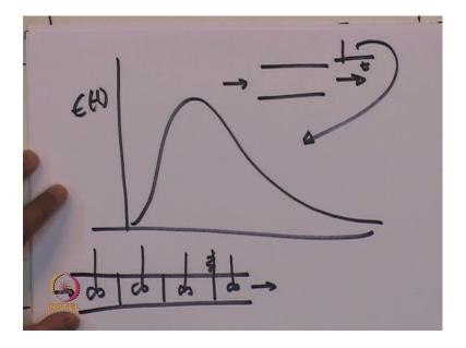
So, let's consider any e curve right once this e curve is obtained, I have a tubular reactor I do a pulse injection experiment and look at an exit age distribution I am going to see this. Now, this is something given to you from this you are going to come up with a model I am going to determine a parameter; now mixing is characterized, by like you have a say let us have a hypothetical mixture or agitator in the reactor.
