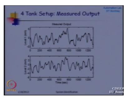
These are the measured outputs we have to measure the outputs again perturbations from the study state level okay, all of these data which means for this particular system I have plate this system I have you know manipulated the valves according to certain.
