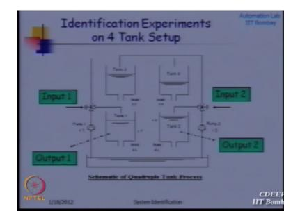
A schematic diagram of the same set up okay and full times where two inputs and I have two outputs, two outputs are still there it is right, and now going to measure all 4 levels and we want to measure only level 1 and level 2 in times fall in time to okay.
