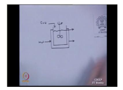
We have this symbol means this is well system okay and it moves out and then there is a jacket here the hitting flow could be stream for example okay some hot fluid in industry they use some hot fluid to let say heat the condense inside this time so the cold stream here and this is hot fluid okay so the cold fluid becomes hot becomes cold there is a exchange of heat between the two and the model for that is.
