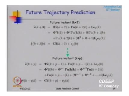
I just go and write in our difference equation. See I have a dynamic model, I can explicitly forecast, so these Z here and Y here are forecast. This is how the system will behave in future, provided I happen to implement, I happen to implement u(k) given K, u(k+1) given K, u(k+2) given K, I can just go on doing this till u(k+p), I can do P step, I had predictions using my difference equation model.
