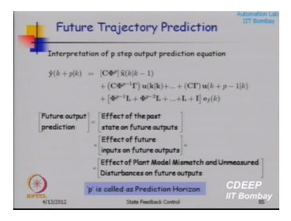
And I want you to understand this very carefully. This prediction P step higher predictions of what is going to happen okay, consist of two components one component is effect of the past on the future, this is the effect of the past on the future, and this is effect of the future on the future. A dynamic system has the memory okay. Let us go back to this painful example of your studies. So x(k) given (k-1) is the current state okay.
