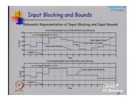
Instead of saying that I am going to manipulate over the entire future horizon, I am going to say that, I am going to manipulate over one input to the next. Then say, I am going to keep the input constant over next three instants, I am going to keep input constant over next five instants, I am going to keep input constant over the prediction okay, instead of changing every input in the future, I am going to constraint the movement in the future.
