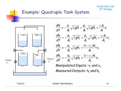
So there is a in a real system there is a way of fixing the ratio flow ratios between the split, so  $\gamma 1$  and  $\gamma 2$  are splits close splits okay, what portion goes to the top time what portion goes to the bottom, yeah.
