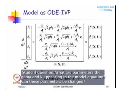
So  $\gamma$  1 and k 1 are the two fix parameters which we can chose the split  $\gamma$  1 talks about the split from to tank 1 and tank 3 yeah, so once you fix it is cost okay.
