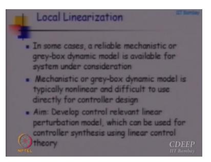
Now so I have model which is available okay now the problem is the model is a non linear differential equation how do I design a controller based on the non linear differential equation it is possible very much possible okay, but the design procedures are very, very cost or very, very difficult as compared to designing based on linear differential equations okay, it is not that we cannot develop the controller using non linear well it becomes very difficult so as a engineer my you know approach.
