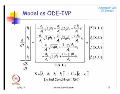
Now what I want to do is I want to develop a linear quadruple machine model starting from this particular model. First of all I am going to classify the variables associated with this model there are two variables or two vectors I am finding out here one set of vectors I am going to call as x okay, this x are dependent variables or states. Here what are the dependent variables, dependent variables how many equations are there, there are four equations, four differential equations.
