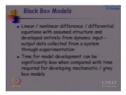
Okay the third category is black box models black box models are non linear difference equations or differential equations with assumed structure what is a structure of this model we have to assume and we will talk about this in great detail how do you develop this models, these models are developed entirely from data we are not using too much of physics are any physics at that for doing this, so this animal is due to u and we will talk about it little later the advantage of this modeling.
