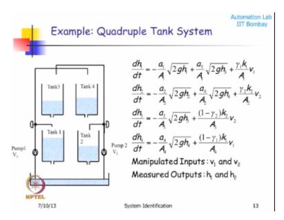
If you look at it has 4 tanks okay here there is a control wall here there is a control wall there are two pumps, the flow here is split okay part of the flow goes to tank 1 part of the flow goes tank 4 okay here the same way on this side part of the flow goes to tank part of the flow goes to tank 3 okay, so this is the interacting systems this is just a toy example that actually illustrates you know what is called as multi variable interactions.
