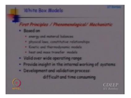
Well that trouble is developing these models is not an easy task typically to develop these models you need an expert, if I have to develop a model for a automobile coming from physics I need a person who understands modeling of automobile you should be a mechanical engineer or a automobile engineer should have done so many courses that you will need to know for doping this modeling.
