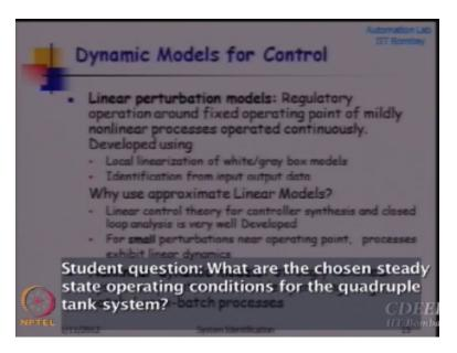
Yeah x bar and u bar yeah, so this is around this p minus conditions this around -p condition h bar is 12.4, 12.7, 1.8, 1.4, u bar is 3 words 3 words okay this voltage is v1 and v2 vary between 1 to 5 or 0 to 5 I have to check in the paper so this is at some middle point okay, the flow ratios have been fixed 2.7 and 0.6 which means 0.7 70% goes to tank one 30% goes to tank 3 and 60% goes to tank 2 and 40% goes to tank 4 so far this condition this particular condition p - conditions okay.
