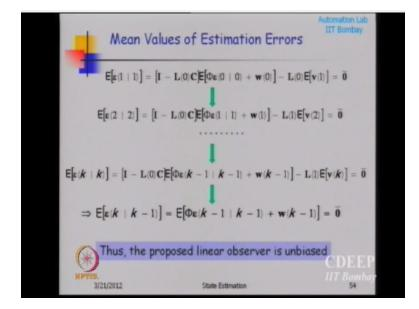
So I am going to start using this equations rolling in time, so now what is the expected value of e 11, will be I - L 0 here x expected value of  $\varphi x e 00$  okay + w 0, what is the expected value of e00 our assumption is that is 0, it is the white noise okay. So what is e 22, see e 22 will depend upon e 1, 1 but e 1, 1 is 0 okay, so what you can show is that, if you make an assumption okay that initial error had 0 mean.
