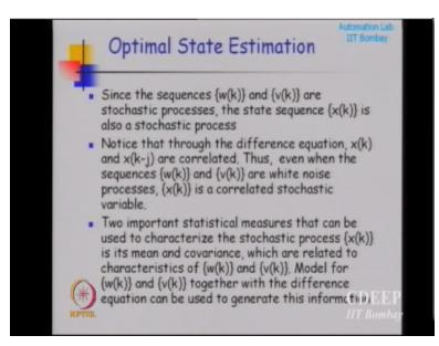
First of all wk and vk stochastic process and by the virtue of the fact that the difference equation is driven by stochastic inputs okay xk is also a stochastic process okay, xk is the function of uk and wk, wk is the stochastic process then the xk is the stochastic process there is the randomness in xk okay. Then this I just talked about that you know through difference equation xk is going to be a colored noise what is the colored noise.
