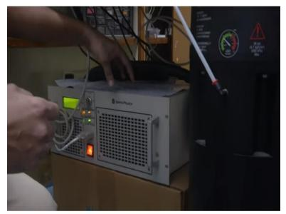
So the whole system starts from down here so where you have array of semiconductor lasers 2 of them 2 bands situated next to each other and driving the converting the electrical power into the light power and those diode arrays are pumped this light into optical fiber which goes through this black cord. This black cord we call it as umbilical it is literally an umbilical because if you had to break this then the whole pump or the whole light power gets terminated and no laser out at all.
