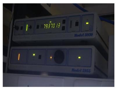
There are two diagnostic modules these are directly read out from the photodiode diagnostics we described in the class. One first here tells you the photodiode output it is right now it is very pretty much full and the other green light that tells you if you read it says pulsing which means it
