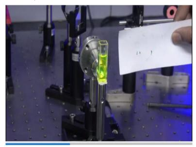
So, now for us to generate the fluorescence okay what we need is that this light coming out right so, the nature of the light that is coming out is collimated right, because we have not put any lens here, so it is a parallel beam of light that is entering into this objective okay. This is an objective lens and we have seen this in the class right, in order to know about the objective lens what we need is; we need to look at these scriptures that are written here okay.
