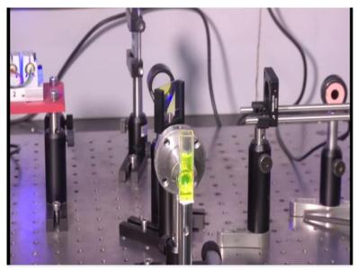
And let us go ahead and see how we actually do that now, just a quick recap; the light source we have; 3 light sources, 3 laser diodes we are operating only the 1; 470 nanometre and that blue light is coming through here hitting this mirror, hitting this mirror and one extra part that we have kept here which is the neutral density filter actually, it reduces the intensity so that it is in a range that it is good enough for us to actually detect and see things.
