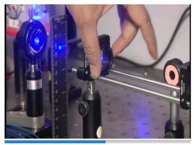
Because the straight line is going like this right, so we did that for the vertical axis and a good test of that is when you actually put in a lens in its path right, please note where the beam is hitting, when you put the lens in its path you should see minimal movement of its position, actually you should not see any movement of its position and that is exactly what you see. So with and without lens you see that the beam nicely makes it through the apertures that we have put in.
