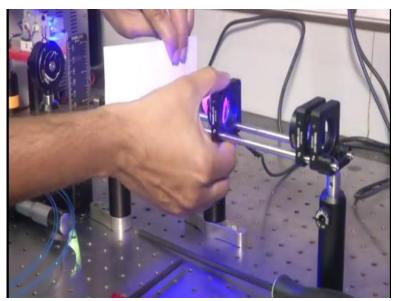
Now, we can actually place the second lens alright, same way and this second lens; this lens is about 35 mm, so as I was telling you in the previous lecture we are putting in this telescope assembly just to ensure not so much of magnification many times you would do it, when we go to infrared beam and ultra-fast laser in setup, we will see that you have to expand the beam.
