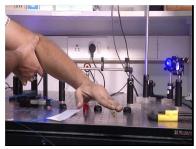
So, first thing you see is that the beam in here is hitting a little bit more on the top edge, then this, so we can actually go ahead and measure where it is actually hitting and if you actually look at it, it is around 5 right, the reading would be around 5 right and here it is a well below 5, it is a 4 and 1/2 or so, so clearly the beam is compared to that is traveling at this direction. So, now and we also know this point where my elbow is right located is also not at the centre of the lens.
