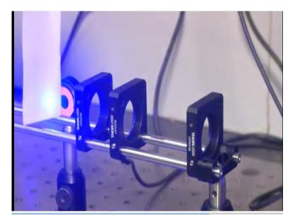
So, we do not want that now that has been ensured by us making sure that the light actually goes through this centre of this cage assembly and we checked it by putting in the lens and making sure it is going through and going through without changing its path.
