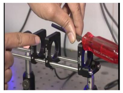
So, now what we are doing; going to do is that align the telescope right, telescope alignment requires that the beam is travelling straight as well as the distance between the lenses alright, are f1 + f2; the sum of the 2 focal lengths okay. So to do that, the cage assembly is really; really helpful even the rails are very helpful why; because as we can see this is called as a cage assembly because this is slightly different from the post, post holder assembly thing.
