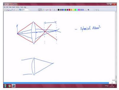
The one of the fundamental assumptions about we writing down the expression for the focal length is that the light incident on the different, different parts of the lens all behave exactly the same, there is not much of a difference. However, that you will see (()) (04:35) is a very strong contradiction to start with itself. The contradiction goes pretty much like this. If you had to assume a point source or then there and it is close by.
