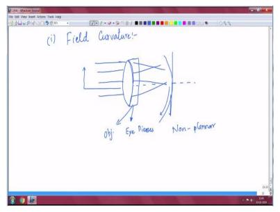
Now apart from this we have is; two other quantities I talked about which is Pin cushion and a Barrel. Oh sorry, before this we need to talk about one more aberration, sorry. It is; this is due to it is called as a curvature, field curvature. So one of the important assumptions that we made is that when we are having an extended object which is not a point object then while; then that
