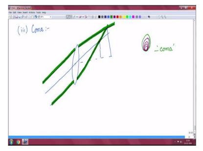
Now the third kind of aberration that we could focus on is Coma. So this originates because of the peripheral race in a lens coming to peripheral rays coming to focus at a different art; at a different distance in the focal plane than that of the central beam that is if you were to take a lens. Now let us take three rays. So we have an optic a ray that going through his optical center. Now if the rays originating from the periphery were to converge at a different place along this axis, okay.
