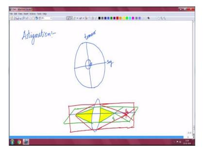
Now next in line of this aberration is our astigmatism. Now this is a result of when we actually look at the lens through. So this is as a result of differential radius of curvature the lens is processing in; or orientation dependent radius of curvature the lenses processing. So to define it let us take two accesses so now do two mutually perpendicular axis, so let us call this as; let us just call this as transverse and let us call this sagittal axis.
