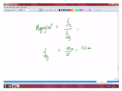
So we were looking at how do we estimate the focal length of the objective and then said what does it mean I mean where does that mean from where do I measure this focal length of the object okay.
