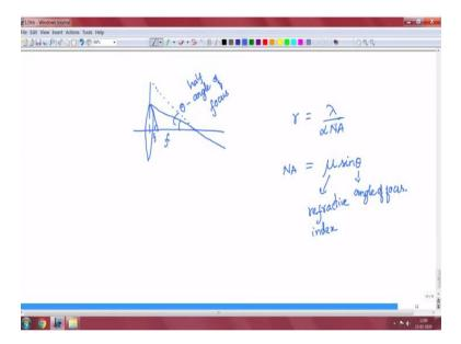
When you keep a sample close to it right or any lens for that matter. So the lens is actually focusing the light beam with an angle theta okay. So we will call this is called as angle of actually half angle of focus but. So now if you have to, I mean we know this that for a given this is a focal length right. So for a given focal length the angle of focus alright the angle of focus if you want to increase you need to increase the size of the objective lens itself or size of the lens.
