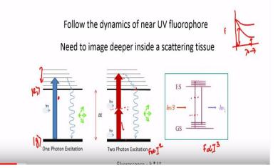
The conclusion was that in any of these, in this or this, any of this, the characteristic equation that describes fluorescence as a function of excitation intensity, would be F directly proportional to I to the power n, by the fluorescence K into i to the power n, so this is a very conclusive evidence to say that you are actually looking at photon process. You are actually looking at two photon excitation and fluorescence.
