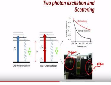
So, now what you see here is that we have seen this fluorescence before right, so we are focusing it down using two lenses, lens one here and then another lens, so inside this we are coming in with 488 nanometer laser, while here we are coming in with 900 nanometer laser, and what we are actually looking at is that when we focus, you will see this will be capable of eliciting one photon fluorescence and in fact you see that result, right.
