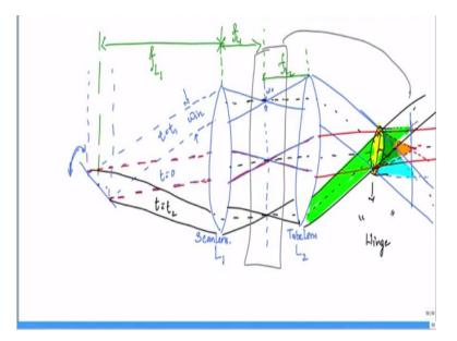
So, now you can actually see how we can actually create a hinge point about the objective lens, so now let us see, you have a mirror that is actually and let us say, the incoming beam is a collimated beam, so now this is a galvanometric mirror so, it is actually going to the axis about which it is going to rotate is coming out of this board and into this board that is about that you are actually rotating, oscillating.
