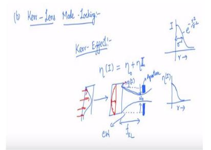
And that is called it is called Kerr lens mode locking. You do that by, this makes use of the idea or an effect called as the optical Kerr effect. So when you look, we had looked at the transfer section of the laser beam. We said that there are different possible modes of this transfer section TM 00, TM 01 and so on and so on.
