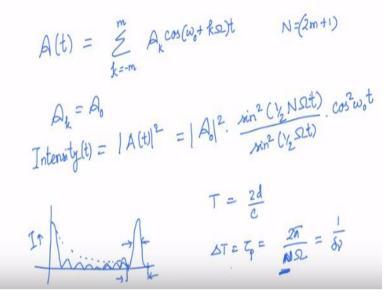
So then what we do is that the next thing is to say the amplitude the resultant amplitude at any time t is given by of the electric field itself right. So k going between 0 to n and for convenience sake what we are going to do is that we are going to split that n into in symmetric interval about 0. So I am going to say m to m such that our total N is basically I mean is covered by this, okay?
