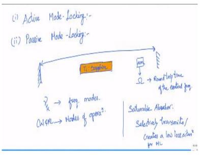
There are two ways of generating these pulses. One is called as active mode locking. And clearly the other is called as passive mode mocking. The active mode locking is a scenario where you are actually having the titanium sapphire. I mean I am going to take an example of a titanium sapphire because that is predominantly what we will be using in the course during our lab demonstration, as well as for understanding the or for utilizing that to in our various microscopic studies.
