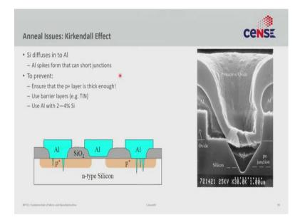
When you deposit aluminum on silicon and heat the system to say 400-500°C or 600°C, not only do you form a silicide, but you also get spikes.
