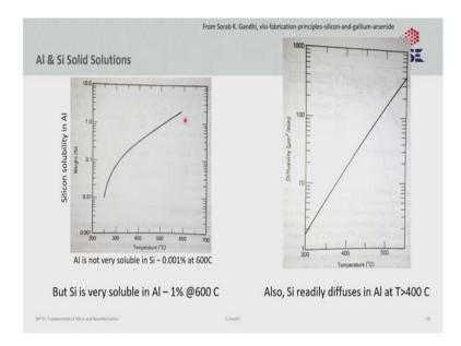
Till now, we looked at the solubility of the metal or a dopant or an impurity into silicon. If you want to analyze how much aluminum diffuses into silicon, you look at the solubility of aluminum in silicon. However, diffusion is a two-way street. Aluminum diffuses into silicon, but silicon might also diffuse into aluminum. After all, there is a gradient there too. So, you must also look at the solubility of silicon in aluminum.
