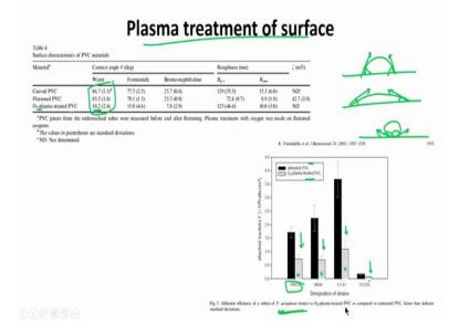
And, then here is another example which is plasma treatment of the surface. So, this is to make it more hydrophilic. So, when you treat a surface of the plasma it becomes oxidized. And, the hydrophilicity of the surface increases, the hydrophobicity goes down and this is what it is showing here. So, you have 3 different surfaces you have a curved PVC, you have flattened PVC and you have O2 treated PVC. And, here they are showing about the water contact angle.
