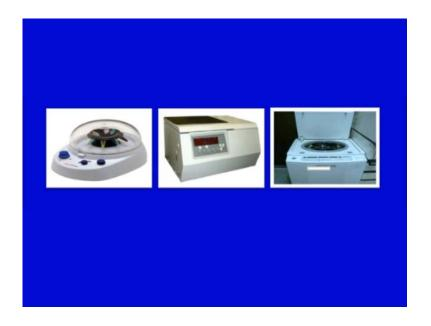
So, you can see here. There are some examples of very small micro centrifuges or micro fuse, you can say a quick spin type centrifuges. There is a table top centrifuge, which is a refrigerated centrifuge. These are little higher floor model centrifuges. So, there could be various kinds of centrifuges for various kinds of applications with lot of flexibility.
