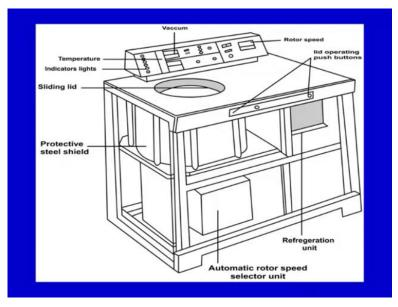
As you can see, there are lot of different things, which are important in here. There is an arrangement for vacuum. You can use switches or these are like controls for vacuum, temperature, indicator lights, and rotor speed. Here, these are lid operating push buttons. Then there is automatic rotor speed selection unit is here. There is a protective steel shielding.
