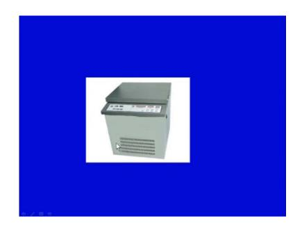
This is typical high capacity refrigerated centrifuges as you can see. This can carry like 4 to 6 litres of material. These could vary in capacity and various types are available in this range. So, we move onto high speed refrigerated centrifuges. Now, high speed refrigerated means they could go to a very high speed. Maximum speed could go approximately up to 25,000 revolutions per minute.
