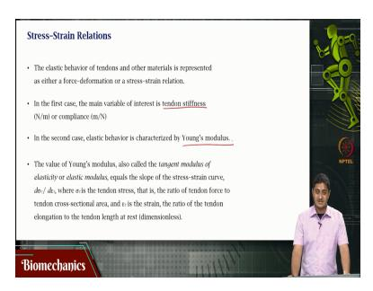
So, as we discussed previously stress strain relations of biological materials, as with engineering materials that represented either as a force deformation curve or also relationship between stress and strain. Essentially the elastic behaviour of these are determined by the relationship between the stress and strain or force and deformation, we have seen this previously. So, if you are looking at a force deformation curve the important variable of interest is stiffness or complaints.
