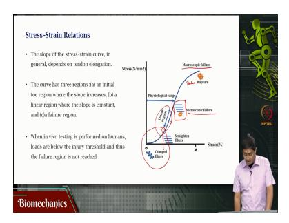
Unlike engineering materials, for a tendon the slope of the stress strain curve in general is a function of the defamation of the tendon. So, that means very clearly that this is not an elastic material, so this is not going to have a modulus. Why? Because the slope of the stress strain curve is the modulus if the slope is a function of the deformation that means what, it is not the force that is a function of the deformation.
