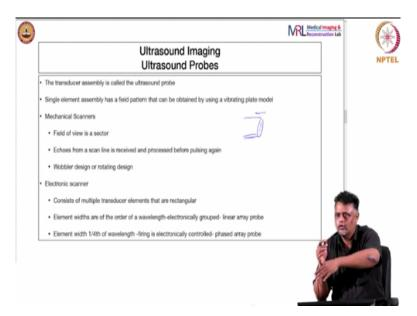
The transducer assembly is called the ultrasound probe. So, it is not like yeah, this crystal like bear and walk around with it, like we will have to put it inside a assembly and it is called ultrasound probe. That is what you see people using when you do an ultrasound scan.
