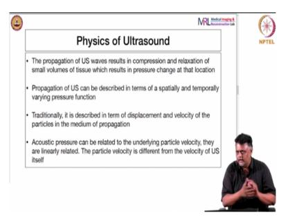
So, why is it the longitudinal wave etcetera? So, it is, the way it generated and wave propagates it is, it is propagates by compression and relaxation of small volumes of tissue. And also it depends on the elastic properties and inertia of the tissue.
