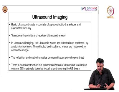
So, as a basic ultrasound system, you know, it consists of a piezoelectric-transducer and associated circuitry. So, we will look at what these are, as we progress through the slides. So, the transducer is the important part of the system it transmits and receives ultrasound energy. We will look at what ultrasound means also in the later slides. And the transmitted, when they say transmitted it transmit them to the human body.
