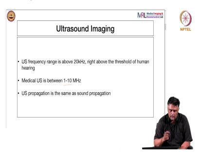
So, what is ultra sound, any frequency sound frequencies sound, just like SONAR. But the frequency range about 20 kHz, but for medical ultrasound is between 1 to 10 MHz. So, the ultra sound propagation is the same as sound propagation. So, all the physics that you use to describe sound propagation can be used here to typically what it is used.
