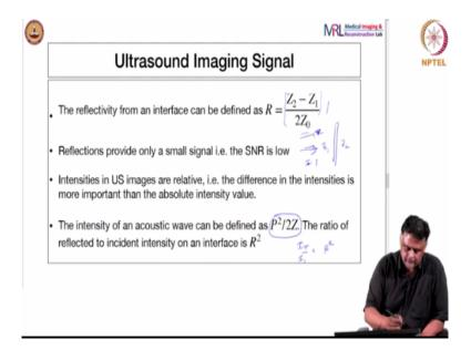
So, the reflectivity then can be defined in terms of the acoustic impedance between let us say, here I am calling Z2 - Z1 is where I have like an interface. There is no here, it is Z1 here it is Z2, there is an incident beam, and it is reflected. So, the reflectivity, or the fraction that is reflected, if you can call it that is the ratio of this. So,  $Z_0$  is an average impedance, like I call it (Z1 + Z2)/2. That is how it is.
