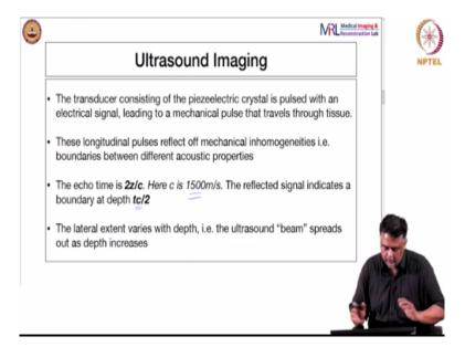
So, here is what I had said before is a transducer which consists of a piezoelectric crystal is pulsed with an electric signal. Because of this pulsing, it starts to vibrate mass fast
