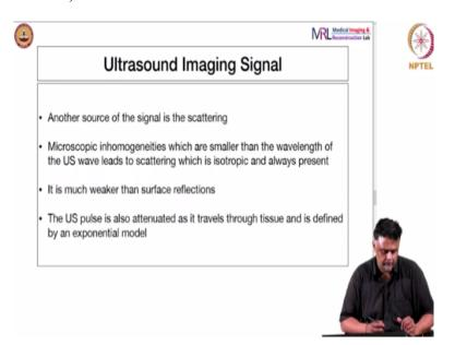
So, there are two, like I said, there are two sources of the signal major sources for the ultrasound signal that you receive. One is the reflection, the other is a scattering. There are always microscopic inhomogeneities in our tissue, these are smaller than the wavelength of
