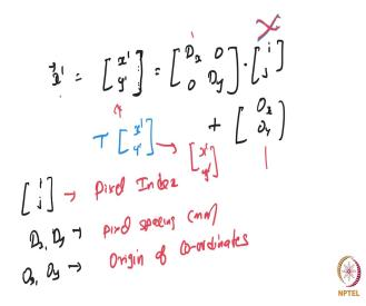
So, there is x', we want to go to, in this case, this is a vector, I write it as x', y'. So, you are going from the index to the coordinate, you have this  $(D_x,0,0,D_y)$  times (i,j), so this is your pixel index. There is a plus  $O_x$ ,  $O_y$ . So, this is (i,j) is your pixel index. That is typically how you would access the elements in an image array. So, this  $D_x$ ,  $D_y$ , or basically your pixel spacing, typically these are in millimeters.
