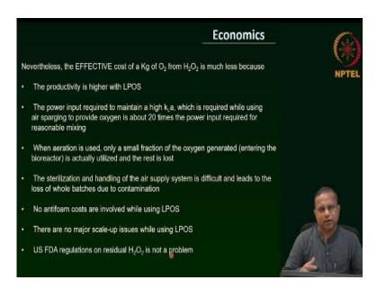
The effective cost of a kg of oxygen from hydrogen peroxide is much less because the productivity is higher with LPOS as we have already seen we have shown that in 15 systems by that by the time the power input required to maintain high  $k_L$ a, remember volumetric mass transfer coefficient high  $k_L$ a which is required while using air sparging to provide oxygen is about 20 times the power input required for a reasonable mixing.
