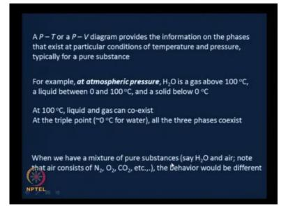
We had already mentioned this: a P-T or a P V diagram provides the information on the phases that exist at particular conditions of temperature and pressure, typically for a pure substance.
