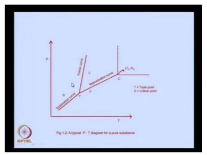
We will take a look at them again here. This is the P-T diagram. Of course, this is only for a pure substance, which mean only one type of substance. We need to interpret this as we saw earlier, as the space consisting of certain values of temperature and corresponding values of pressure. This is the sublimation curve, which is essentially a demarcating line between the region where the solid exists and the vapour exists.
