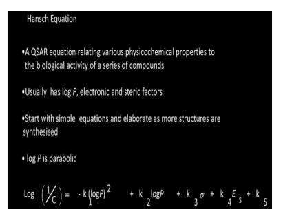
Then comes Hansch equation, what is Hansch equation A QSAR equation relating various physicochemical properties to the biological activity of a series of compounds. So, you will have log p coming into picture electronic factors coming into picture steric factor. Okay So we can have a QSAR activity on the left-hand side which may have terms related to electronic, steric and log p.
