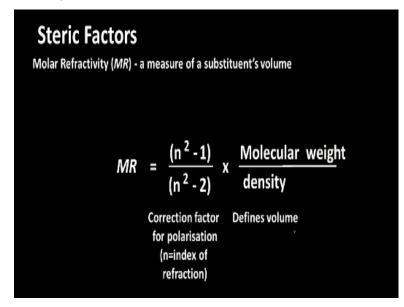
You also have a term called Molar Refractivity it is a measure of substituents volume this is a descriptor which we can calculate that is called Molar refractivity it is given by n square-1/n square-2 molecular weight/density okay this is a correction factor this is called index of refraction correction factor for polarization okay it is called index of refraction. So, it is a function of molecular weight function of density that is called Molar Refractivity.
