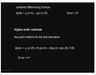
There is another method that is called centered difference formula. That means you do x+h, x-h and then divide by 2h, okay. So, this is x+h and then we have the x we have the x+h here we have the x here and suppose we have x-h here, okay. So, you calculate at x-h, so this difference will be 2h, okay, so this is at a function of xh and this is at a function at x-h and the difference is 2h.
