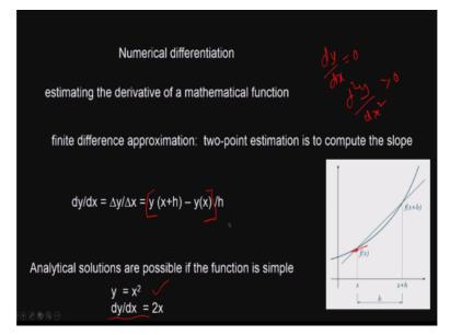
Because like I mentioned if you are going to look at minima then we need to think that dy/dx should be = 0 and d square y/d x square should be > 0. So, dy/dx is calculated, okay which we looked at in the previous class, okay. So, we need to understand how the computer is use numerical techniques to calculate that. If it is in analytical solution, then it is quite simple. For example, if you have y=x square, so dy/dx = 2x.
