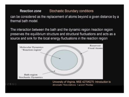
Reaction zone, this can be considered as a replacement of atoms beyond a given distance by a thermal bath model, so we have the reaction region, we have the stochastic dynamics here, you have fixed amount of atoms here okay, the interaction between the bath and the dynamic region, reaction region preserves the equilibrium structure okay, and then this reservoir okay, maintains the energies these solvent molecules face actually okay.
