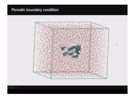
This is the protein, this is the periodic box, we have assumed it here okay, a large cube like, there are lot of water molecules here and so we assume similar boxes on all the 6 sides of this cube so we can perform molecular dynamic simulations we can perform conformational changes so if one water molecule goes out from this box to the box outside it is assumed another water molecule will enter.
