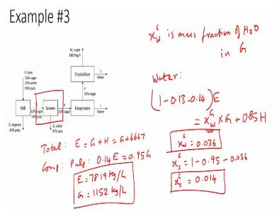
Now that we have calculate the streams L, K, J and H we can start with the system of stream to identify the mass flow rates of E and G. So for starting that let us first write the total balance equation. The total balance equation for this stream would be E = G + H and then we can write component balances here we would choose pulp as the component balances because we know the concentration of pulp in the input stream E and exit stream G.
