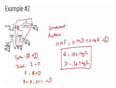
We do not have the composition of this particular stream as we do not know the composition or the mass flow rate of the stream it would be very difficult to estimate what this particular stream would be. Thankfully the problem does not expect us to calculate the stream so instead of trying to identify this particular stream we can now choose a system which would be basically (()) (06:40) the stream how would we do that?
