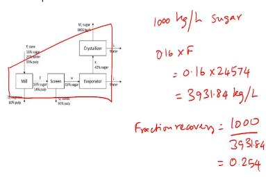
Now we need to perform similar calculation to identify the flow rate and the composition of the gas stream which is the stream D how we go about that we identify nil as the system and once we have identify the millers the system we need to understand that we have all the information about the system which is the cane stream which is the feed stream is entering into the mill we have all the information.
