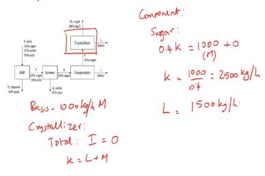
So let us look at one last example problem before we conclude this particular topic. So here the figure shows the process for extraction of sugar and sugarcane all the known data is given here we asked to calculate the composition of every flow stream and the fraction of sugar in the cane that is recovered so to do this we need to get the information about the all the unknown streams.
