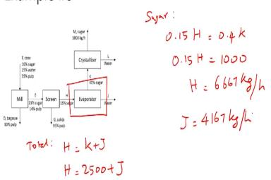
So now we have identified one system and solve the balances for K and L so similarly we can now choose the next system which would be the evaporator. So for this stream again we have the information about the stream K and the information about stream J and the information for also given. So we have the composition for all the three stream however the mass flow rate is known only for the stream K.
