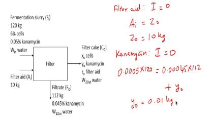
We can continue writing component balances for filter aid we can write the component balance as again input = output so the input comes only through AI and output leaves only through C naught so the amount of filtering leaving the system through the filter cake which is written as Z naught. So AI = Z naught implying Z naught would be 10 kilograms. So we can still write a balance equation for kanamycin and for water.
