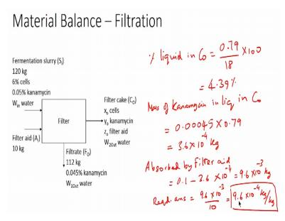
Now the next balance equation we can write would be the water balance again input = output so input is through water is coming in through the slurry so we would call that W in = W 1 out + W2 out. Water is entering into the system through the fermentation slurry it has been given that the concentration of kanamycin in fermentation slurry is 0.05% and the concentration of cells in the slurry is 6% so the rest as to be water.
