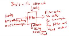
Let us now look at an example problem for filtration a fermentation containing Streptomyces kanamyceticus cells is filtered using a continuous rotary vacuum filters 120 kilograms per hour slurry is fed to the filter 1 kilogram slurry contains 60 grams of cell solid to improve the filtration rates particle of diatomaceous earth filter aid are added at a rate of 10 kilograms per hour.
