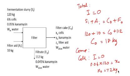
So knowing all these information let us go about solving this problem here is the flow chart which we drew so in more legible fonts. Now let us start with the balance equation so the first balance we write either total balance the total balance equation for this system the total balance equation for this system would basically be input = output because it is the system is in steady state leading to accumulation be 0 and ask the system does not have any reaction happening.
