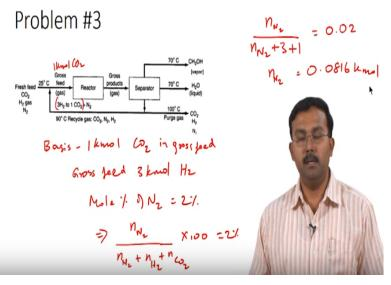
Based on the information given to us in the problem we can use the basis as 1 kmol of CO2 in gross feed. So we have been told that 1 kmol of CO2 enters into the reactor. So which means this is the gross feed and you have 1 kmol of CO2 entering here. So this is the basis given. So we have also been told that the feed which is entering the reactor contains stoichiometric ratio of CO2 and hydrogen which is 3:1 so which is also been given to us.
