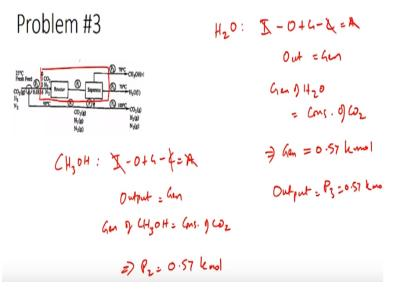
So we also need to identify how much of methanol and water are leaving the system which we had chosen. The system we had been working on is this, which is the reactor + separator. So to identify the amount of methanol, we have to write a methanol balance. So methanol balance would be input - output + generation - consumption = accumulation. At steady state accumulation goes to 0 and methanol is not being consumed as it is a product.
