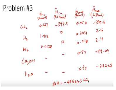
Now that we have calculated all the enthalpy values, let us go ahead and fill the enthalpy table. So the enthalpy table which we had was CO2, hydrogen, nitrogen, methanol, and water. So we had n in dot, H cap in, n out dot, and H cap out. So the values for n in and n out are 0.637 kmol, 1.913 kmol and 0.0128 kmol. So please note that these values are all in kilo moles and the values for H cap we calculated were all in kilo joules per mole.
