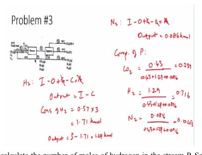
We now have to calculate the number of moles of hydrogen in the stream P. So using the same system, we need to now write a hydrogen balance. The hydrogen balance again is input – output + generation – consumptions = accumulation. At steady state there is no accumulation. Again, hydrogen is a reactant so there is no generation of hydrogen. So your output again would become input – consumption. So input we already know is 3 kmol. So what is consumption?
