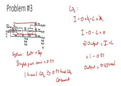
For using this value, we need to ensure that the reactant which is entering the reactor only passes through the reactor a single time. So which means we have to take the reactor, the gross feed as the component which is crossing the system boundary and we need to ensure that whatever is leaving does not come back through the recycle stream and the system needs to be chosen appropriately.
