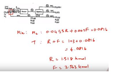
Now to get the information on the fresh feed and the recycled feed, we need to choose a different system. So here we could use the mixing point as the system. So if we were to use mixing point as the system then we can actually write two different balances. One would be for nitrogen and the other could be for the total balance and using these we will be able to solve for the two unknowns. The first unknown is the recycle amount R and the other is the feed rate F.
