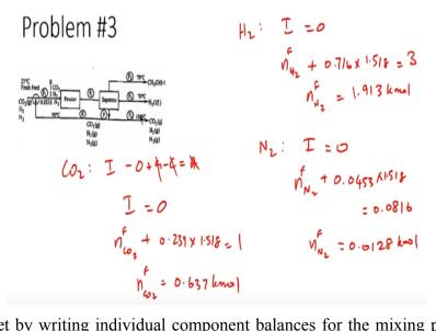
So that we can get by writing individual component balances for the mixing point. Let us now write the carbon dioxide balance for the mixing point. It would be input – output + generation – consumption = accumulation. So no accumulation at steady state. No generation or consumption. It is a nonreactive system. So input = output. So your input actually has two terms. One is through the fresh feed. Other is through the recycle feed.
