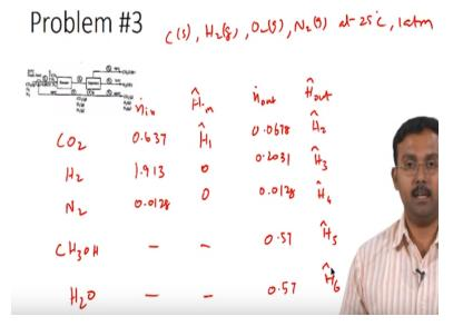
So let us build the enthalpy table for the overall system. So the overall system encompasses the mixing point, reactor and the separator. So the only streams which are crossing the system boundary are the fresh feed which contains carbon dioxide, hydrogen, and nitrogen and you have the product streams which are methanol and water and the purge stream which contains carbon dioxide, hydrogen, and nitrogen. So let us now write the enthalpy table for this.
