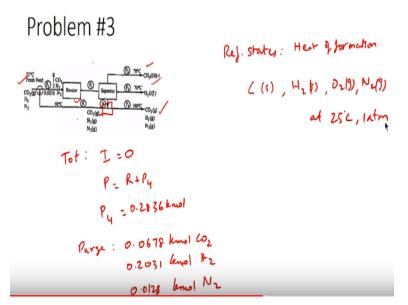
So for doing that we will have to write a balance for the splitter as we now have the information about the fresh feed. We have information about the recycle stream. We have information about P 2, P 3. We just need to get the information about P 4. For this we can write the total balance equation for the splitter. The total balance for the splitter would just be input = output and input is actually P. This is = R + P 4. So solving for this we will actually get P 4 = 0.2836 kmol.
