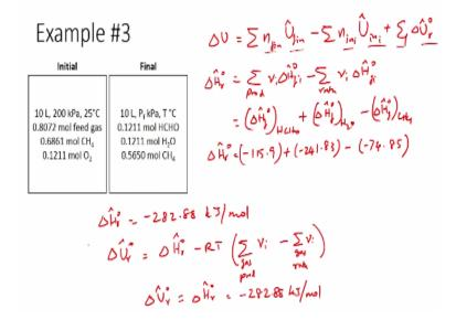
To calculate the change in internal energy delta U, we need the internal energy of the reaction as well. So delta U would actually be equal to sigma of n final times U cap final – sigma of n initial times U cap initial + the psi which is extent of reaction times delta U r which would be the internal energy of reaction. So here we already identified the internal energy of the final and the initial conditions using the polynomials we have.
