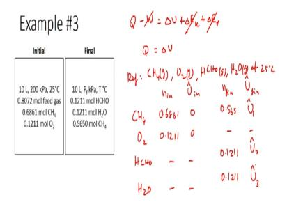
Now that we have performed all the required material balances, we can start with the energy balance calculations. Here it is a closed system unlike all the systems which we have been looking at till now. For a closed system the equation would be Q - W = delta U + delta E k + delta E p. So here there is no change in kinetic and potential energy and there are no moving parts so you have work also = 0.
