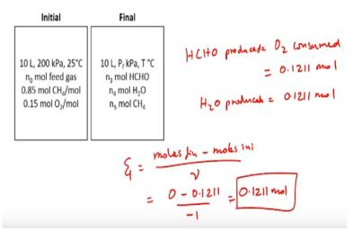
So we also need to identify the number of moles of formaldehyde and water which is present. Based on the stoichiometry for every mole of oxygen consumed 1 mole of formaldehyde and 1 mole of water is produced. So you can calculate formaldehyde produced would be equal to oxygen consumed and this would be 0.1211 moles. Similarly, water produced would also be equal to 0.1211 moles.
