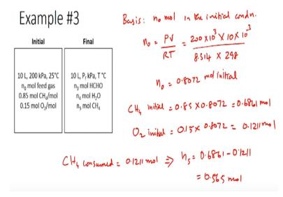
Here is the example problem in terms of the flow sheet. You have an initial and final condition. It is a closed system which is 10 L, 200 kPa and 25 degree Celsius in the initial condition. It contains n naught moles of feed gas and you know the composition of this feed gas. Initial condition is 0.85 moles of methane and 0.15 moles of oxygen per mole of the mixture.
