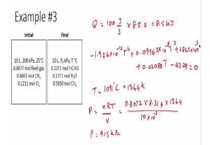
So in the problem statement, we have been told that heat is supplied by an electric coil at a rate of 100 watts for 85 seconds and then it is stopped. So the amount of heat which is supplied would be Q = 100 J/s times 85 s. So this would give us in terms of joules which is 8500 J or 8.5 kJ. So the total amount of heat supplied would be 8.5 kJ. So we have all the terms. So we have a polynomial representing the change in internal energies.
