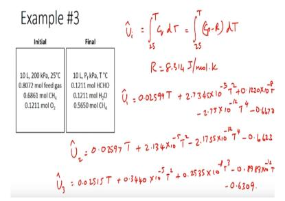
So we know that U 1 cap would be equal to integral 25 to T C v dT. So we have always been using C p. So we will use C v here. So if it is solid or a liquid, C p will be roughly equal to C v. However, here everything is a gas. For a gaseous system you would have C p = C v + R. So you will calculate C v as integral 25 to T C p - R dt. So C p value is readily available from your tables and from textbooks and reference books.
