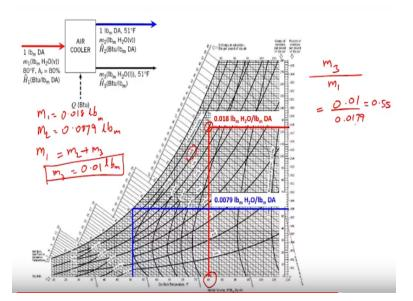
So we are assuming that 1 pound mass of dry air is actually entering into the system and this contains m 1 pound mass of water vapor which is because it is 80 degree Fahrenheit with a relative humidity of 80%. It enters into the air cooler and it gets cooled where some of the water condenses and leaves and the other rest leaves as the air water mixture which must be the saturation air water mixture at 51 degree Fahrenheit.
