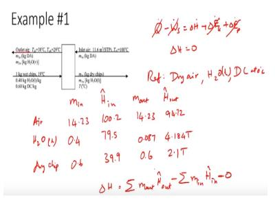
For the next part of the problem, we are asked to identify the temperature at which the wood chips would be leaving. So for identifying that we would have to perform energy balance calculations. So here all the required material balances have been done. So we will start with identifying what the equation would be. So this is an open system which means the general energy balance equation would have enthalpy instead of internal energy.
