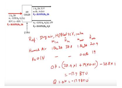
Now that we have all the masses and enthalpies for the inlet and the outlet stream we can perform energy balance calculations so that we can get the amount of heat that needs to be removed or Q. So how do we do that? So first we again have to build the specific enthalpy table. So for that we will have to identify the reference states. As I had mentioned the reference state for the psychrometric chart is dry air and water at 32 degree Fahrenheit and 1 atmosphere.
