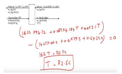
14.23 times 94.72 + 0.087 times 4.184 T + 0.6 times 2.1 T. This is the total enthalpy of the outlet streams minus the total enthalpy of the inlet streams which would be 14.23 times 100.2 + 0.4 times 79.5 + 0.6 times 39.9 = 0. So with this the equation comes down to 1.62 times T = 133.72. So T = 82.3 degree Celsius. So the temperature of the wood chips which are leaving the system is 82.3 degree Celsius.
