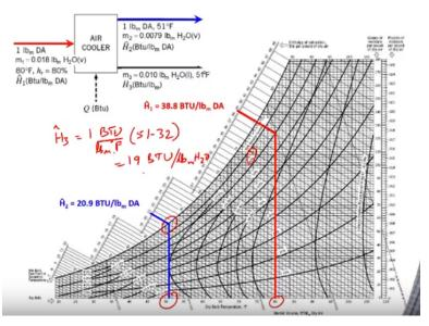
Now that we have identified the masses of water vapor coming in, water vapor leaving and water liquid leaving, we need to identify the enthalpies of the inlet and outlet streams. So the inlet stream you have air water mixture coming in at 80 degree Fahrenheit and 80% relative humidity so which would mean again we can draw the same line from 80 degree Fahrenheit to 80%
