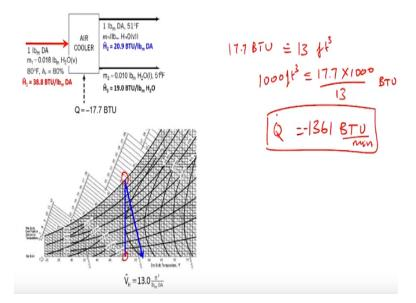
The problem asks us to identify how much of heat needs to be removed for producing 1000 feet cube of humid air. So we know the mass of dry air which is leaving the system. However, we do not have the volume of humid air which is leaving the system directly. So that we can identify using the humid volume data. So the exit stream is at 51 degree Fahrenheit and 100% relative humidity.
