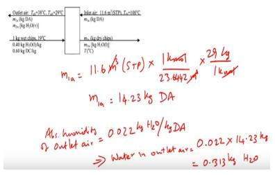
Before we start performing the material and energy balance calculations the first information we need is the mass of air which is entering into the system. So we know that 11.6 meter cube at
