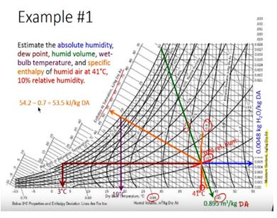
Let us look at a couple of example problems which will help us understand how to read these psychrometric charts to get the different parameters that we looked at. So we have been given a condition of 41 degree Celsius and 10% relative humidity and asked to calculate all the parameters that we had looked at till now. So the first thing we want to calculate is the absolute humidity. For that let us first identify the points which we are interested in. 41 degree Celsius.
