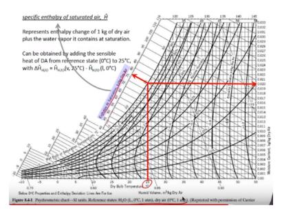
Since these psychrometric charts have to be used for performing energy balance calculations, enthalpy values can also be obtained from here. So for saturated air, you can get enthalpy values directly. You see that enthalpy at saturation listed here and you can calculate the enthalpy at saturation from these graphs.
