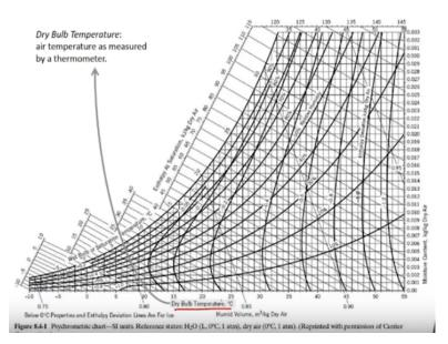
So using these two reference states we have calculated and plotted all this information. So what information is readily available for us from here? The first thing we have is the dry bulb temperature. So the x axis you have here, this is the dry bulb temperature. So this dry bulb temperature basically is the temperature which you would measure using a thermometer. Any thermometer that hangs in an open space would be able to measure the dry bulb temperature.
