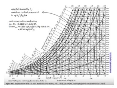
So absolute humidity is basically measured in terms of kilograms of water per kilogram of dry air. So this needs to be clearly understood. The denominator is kilogram of dry air, not kilogram of air total. So total air would contain water vapor and dry air. So that would be called the moist air. So here we are looking at the kilograms of the mass of water vapor which is present per kilogram of dry air.
