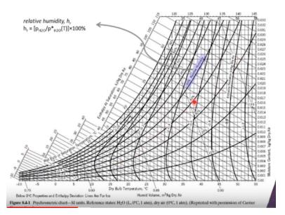
So the next information you can get is relative humidity. So relative humidity is basically the ratio of partial pressure to the vapor pressure times 100 for a given temperature. So this gives you the information about what is the relative level of humidity compared to saturation conditions. So for any temperature there is only so much water vapor that can be present in equilibrium along with air until it starts condensing. So that is the saturation condition.
