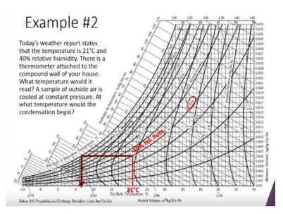
So we will look at an example problem which has everyday applications. Today's weather report states that temperature is 21 degree Celsius and 40% relative humidity. There is a thermometer attached to the compound wall of your house. What temperature would it read? A sample of outside air is cooled at a constant pressure. What temperature would the condensation begin at? So the first point we need to look at is we have a thermometer hanging out and we need to know what thermometer it would read.
