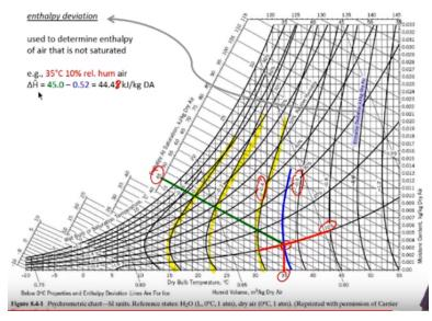
That can be obtained by using the enthalpy deviation curves. So now other than the straight lines which we had looked at and the curves for relative humidity that we have looked at we also have other curves which are shown here. So these are the curves that we have. You see the curves here. So those curves are called the curves for enthalpy deviation. So we can actually calculate enthalpy changes, specific enthalpy for non-saturated air using these enthalpy deviations.
