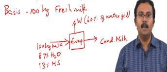
So let us look at an example for a evaporator which would help us understand the fundamentals of performing material balances for the system unsweetened condensed milk is the shelf-stable canned milk product. If 100 kilogram of fresh milk containing 87% water and the rest milk solids is condensed using an evaporator to remove 60% water from the fresh milk you are asked to
