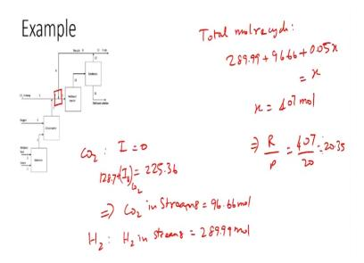
Let us write the balance equation for the mixing point the carbon dioxide balance would be input = output so input is 2 steam 1 is steam 7 and other is 8 and output is steam 9 we know that the output is 225.36 and input in steam 7 is 128.7 and the rest would be the input in the steam 8. So this would be the CO2 input in steam 8 so this would be CO2 steam 8 can be calculated as 96.66 moles.
