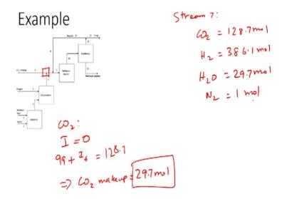
Now that we know 128.7 moles of CO2 is present we can write a balance for a mixing point for CO2. If the CO2 balance for mixing point would be input = output so you have 2 inputs here one input comes from steam 5 which contains 99 moles of carbon dioxide and you have another input from the CO2 make up steam will just call that I6 would be equal to the output which know is 128.7 moles.
