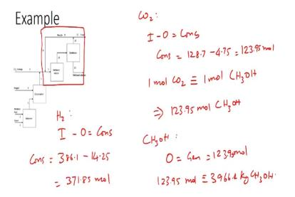
Using this we will be able calculate how much methanol has been produced let us try and do this so if you were to write the balance equation for hydrogen for the system chosen we basically this what you would have is input –output = consumption we already know that input is 386.1 which is coming in through steam 7 and we calculated that the output was 14.25 from the purge steam so consumption is basically = distance between the 2 which is 371.85 moles.
