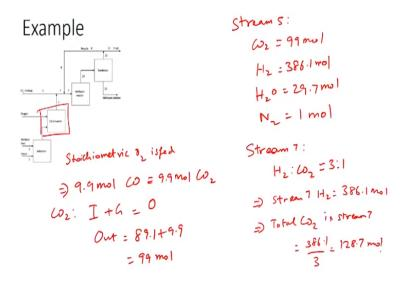
So now we have performed the calculations for the first system the next system of interest would be the CO convertor for the CO convertor we have been told that stoichiometric requirement of oxygen is fed and there is carbon monoxide to carbon dioxide. This implies the 9.9 moles of carbon monoxide gets converted to form 9.9 moles of carbon dioxide. So if you were to write a carbon dioxide balance you would have input + generation = output.
