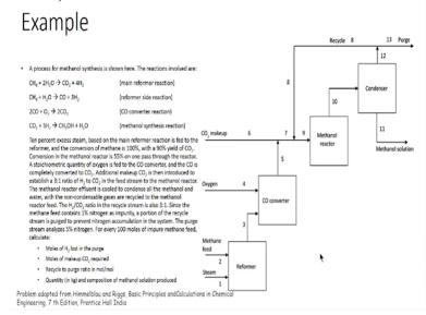
Here is the example problem a process for methanol process is shown here the reactions involved are methane + water forming carbon dioxide and hydrogen methane + water forming carbon dioxide and hydrogen and carbon monoxide + oxygen forming carbon dioxide. And carbon dioxide reacting at hydrogen perform methanol and water.
