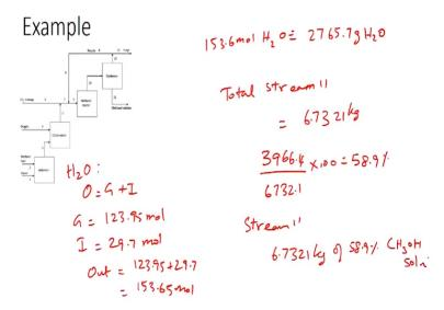
For that we need to perform the water balance equation so the balance equation would again be output = generation + input so using stoichiometric generation would be equal to 123.95 moles of water being produced we already know input is 29.7 moles coming in through steam 7 this means our output for water in steam level would be 123.95 + 29.7giving you a value of 153.65 moles.
