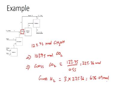
For calculating the recycle steam we would like to write a balance equation for either the mixing point or for the splitting point the problem with the splitting would be we would have only one independent balance equation so it is better to write the balance for the mixing point so for writing the balance for the mixing point we would have to have information about steam line. How do we get information about steam line?
