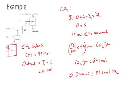
Let us try to solve this problem the problem statement gives us that 100 moles of impure methane is fed which means stream 2 would contain 100 moles which would be 99% methane and 1% nitrogen given as 99 moles of methane and 1 mole of nitrogen in stream 2. So our base is would be 100 moles in stream 2 so this contains 99 moles of methane and 1 mole of nitrogen so we have also been told that stream 1 is 10% excess water vapor which is being fed or steam which is being fed.
