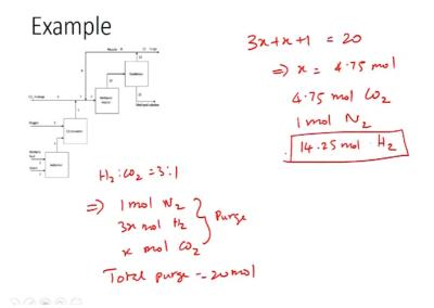
So what we have here is hydrogen is to carbon dioxide in purge steam is 3 is to 1 this implies you have 1 mole of nitrogen 3X moles of hydrogen and X moles of carbon dioxide in the purge steam. The total purge is calculated already as 20 moles so what we can do is 3X + X + 1 which is the total number of purge steam = 20 giving you X as 4.75 moles.
