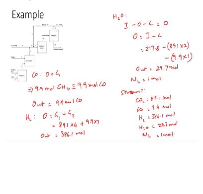
Similar to carbon dioxide we can also perform carbon monoxide balance which would again be output = generation so we knew that 90% of methane which was consumed went into main reformer and the rest 10% went into side reformer reaction this implies 9.9 moles of methane went into formation of carbon monoxide based on stoichiometric this would have produced 9.9 moles of carbon monoxide.
