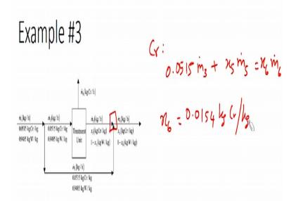
For the mixing point we can also write the chromium balance the chromium balance for the mixing point would be 0.0515 times M3 dot + X5 times M5 dot = X6 times M6 dot. We already know M3 dot M5 dot M6 dot and also X5 so substituting the values we would get X6 which would be 0.0154 kilograms of chromium per kilogram. So with that we have come to the conclusion of example problems related to systems with bypass.
