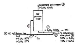
So here is an example problem in the feed stock preparation section of the a plant manufacturing natural gasoline isopentane is removed from butane free gasoline. The process and the components are shown here that fraction of butane free gasoline is passed through the isopentane tower. So what you have here is a feed of 100 kilograms of butane free feed and that enters into the isopentane tower.
