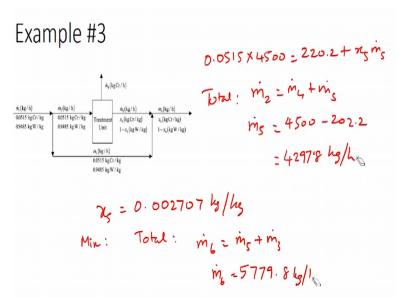
So writing the total balance for treatment we would basically have substituting this M4 dot into the chromium balance we would have 0.0515 times 4500 = 220.2 + X5 M5 dot. So we can also write the total balance for the treatment unit which would be M2 dot = M4 dot + M5 dot so we already know M2 and M4 so we can calculate M5 as 4500 - 202.2 giving you a value of 4297.8 kilogram per hour.
