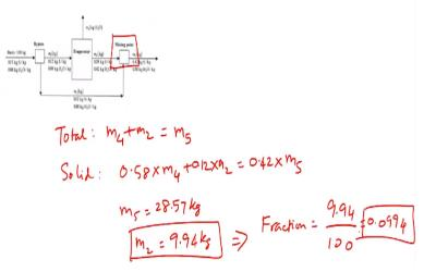
So for the mixing point let us try to write a balance equation for this mixing point. So the total mass balance for the mixing point would be M4 which is the mass enteing through the
