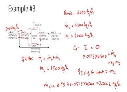
So here we have the flow chart and now we try to solve the material balances so that we can calculate the mass flow rates. So we have been told that the basis to be used for our calculations is 6000 kilograms per hours which is being fed. So this M1 dot would be 6000 kilograms per hour so this means only 4500 can actually enter into the treatment unit. So M2 has to be only 4500 so we know that M2 dot = 4500 kilograms per hour because that is what the treatment plant can handle.
