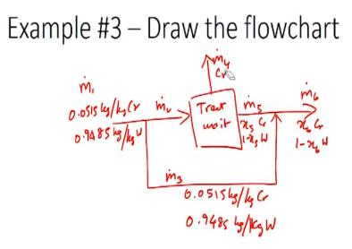
So what we have is a stream which contains 5.15% chromium is actually being sent to a treatment unit. So let us call this as treatment unit so from the treatment unit 95% of chromium is recovered and recycle back into the plant. The rest of the fluid is sent back to sent to the waste lagoon as waste treatment for as waste which is being discarded. So this treatment unit has been designed to handle only 4500 kilograms per hour of the liquid.
