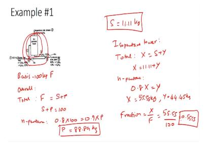
The first step for any material balance problem is to identify the basis in these problem 100 kilograms of butane free gasoline is being fed to the system which means the basis would be 100 kilograms of butane free feed. So we will use the basis as 100 kilograms of F so we can identify different system for performing material balance calculations.
