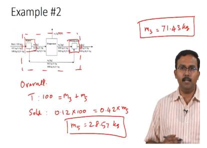
As I had already mentioned the basis is 100 kilograms and now this is important for us to identify which system we want to work with. So as always we will start with the overall system as always we will start with the overall so the overall system would encompass the bypass stream.
