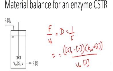
So now we have the definition for F by VR as dilution rate so this is a term which is usually used for understanding and designing reactors so this dilution rate is equal to 1. tou which is the residence time inside the reactor. So we can calculate the residence time Tou as S naught – S times KM + S divided by VM times S. So using this equation we can calculate the residence time for the reactor and also we can calculate the volume of the reactor to design the CSTR for the required operations.
