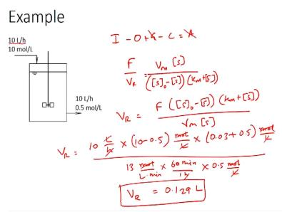
So the first step would be to identify the basis so here we have been 10 liter per hour is the inlet feed of the subset so we will take that as the basis with that we can write material balances which would be input – output + generation – consumption = accumulation at steady state there is no accumulation as we are writing the balance for the substrate the generation would also be 0.
