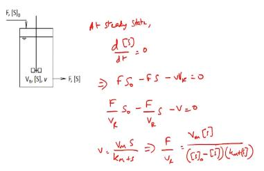
So from here we can assume certain condition such as steady state and thereby at steady state you have DSDT = 0 so this implies the equation becomes S naught – FS – VVR = 0. So dividing the entire equation by volume of the reactor we get F by VR times F naught – F by VR times S – V = 0. From the MICHAELICS MENTEN equation we know that V = VMS divided by KM + S.
