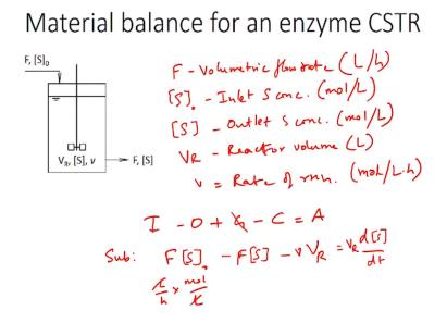
So this represents a CSTR with all the parameters listed now so here you have F which is volumetric flow rate so which would be in terms of liters per hour and you would have S naught which is the inlet substrate concentrate this can be in terms of moles per liter or grams per liter and you have S which is the outlet substrate concentration again in terms of moles per liter and
