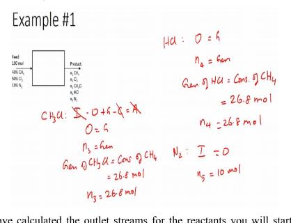
Now that we have calculated the outlet streams for the reactants you will start with the other products which are formed this reaction and also the inert which is entering and leaving the reactants. So now you will write a balance equation for CH3 CL so again we will start with input - output + generation – consumption = accumulation. Accumulation goes to 0 so this is a product so there is no consumption is only generation there is now input of CH3CL.
