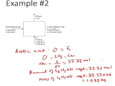
So now that we have calculated the composition of air we now have to move to the first part of the problem where we have been asked to calculate the minimum mass of ethanol required for producing 2 kilograms per hour acetic acid. So for this you will have to start with acetic acid balance so if we start with the acetic acid balance you would end up with output = generation + there is no input of acetic acid.
