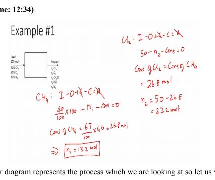
So this particular diagram represents the process which we are looking at so let us write the mass balances for each of the component. So for methane the system would the balance equation would look like input – output + generation – consumption = accumulation assuming steady state accumulation goes to 0 methane is actually taking part in reaction it will just get consumed it will not get generated so generation goes to 0 you have both input and output terms.
