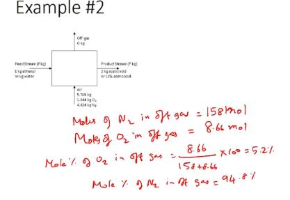
So what we can do for that is convert the mass of oxygen and nitrogen to moles of nitrogen and oxygen. So moles of nitrogen in half gas = moles of nitrogen in the half gas would be equal to 158 moles and moles of oxygen in half gas = 8.66 moles you can perform these conversions to confirm these numbers. So mole percentage of oxygen in half gas would be equal to 8.66 moles / 156 + 8.66 times 100 giving you a value of 5.2 percent.
