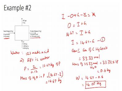
Now we next part of the problem we have been asked to calculate the minimum amount of water that is required for diluting the acetic acid solution so that the percentage of acetic acid is not exceed 12%. So this we need to perform a material balance on water. So let us try and write a water balance equation for that we need to understand the composition of the product stream.
