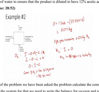
For the last part of the problem we have been asked the problem calculate the composition of gas which is leaving the system for that we need to write the balance for oxygen and nitrogen. So we know that 1.34 % of oxygen and 4.424 kilograms of nitrogen are entering into the system.
