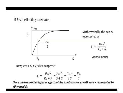
If we consider the limiting substrate and let us say if S is the limiting substrate, then the variation of the specific growth rate mu, remember that r x equals mu x we said,
