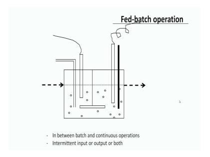
Then a fed-batch operation, which is in between a batch and a continuous operation where there could be intermittent input or output or both, both intermittent output and the intermittent input, at the same time. Some reactors we said, nicely fit into all 3 modes of the possibilities of operating them in all 3 modes of operation, some of them do not. This is think, where we finished up the last lecture.
