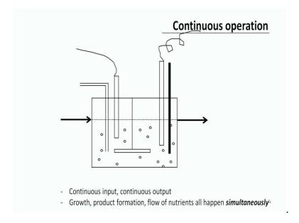
Or a continuous operation, where there is a continuous input, a continuous output. The growth, product formation, flow of nutrients - all happen simultaneously.
