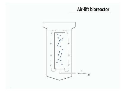
And then an air-lift bioreactor, a Packed bed bioreactor, a Fluidized bed bioreactor - which is nothing but a packed bed which jiggles around.
