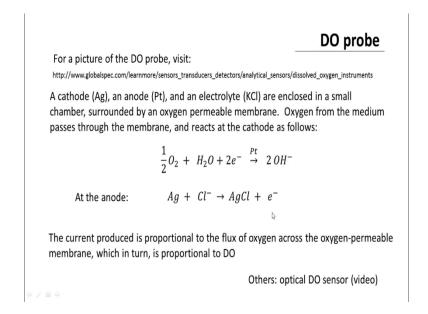
The DO probe, the probe that is used to measure the dissolved oxygen level. For a picture, you could visit the site mentioned in the video. It is an electrochemical probe therefore; you have a cathode which is platinum, an anode which is silver.
